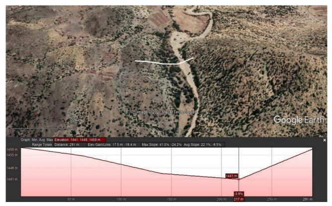
Figure 9. Second location for potential dam site section, showing the location of the section and the dam crest length 0 with 17m crest height.
