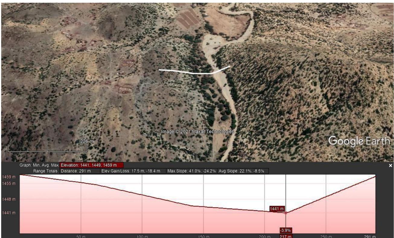
Figure 9. Second location for potential dam site section, showing the location of the section and the dam crest length with 17m crest height.
