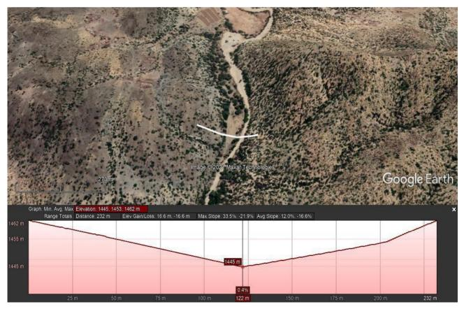
Figure 8. Potential dam site section, showing the location of the section and the dam crest length with 17m crest height 9
