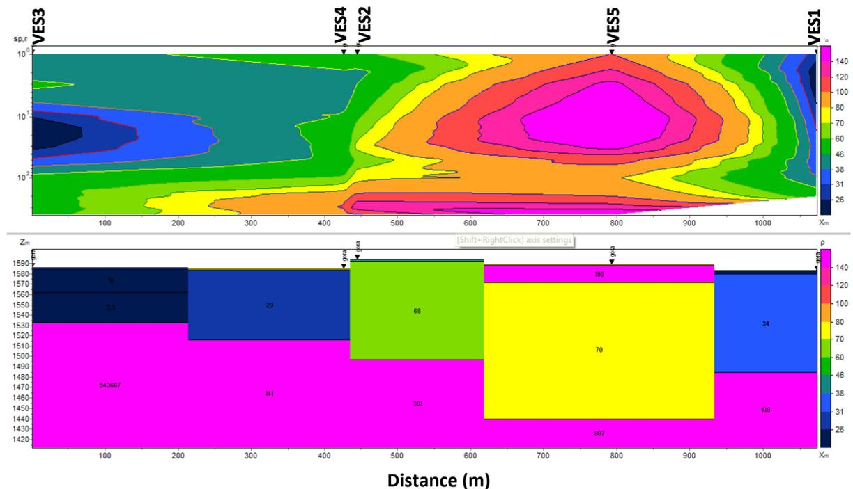
As its can be seen on the above depicted cross section, the location of VES5 was found to have the deepest basement rocks, hence, the location of VES5 is selected as 1<sup>st</sup> priority site to be drilled.
