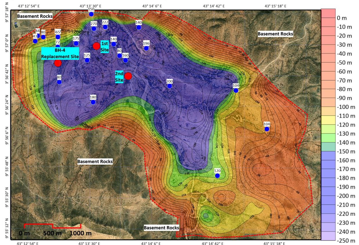
As it can be observed from the above depicted Amoud area aquifer depth modeled map, the two selected sites by SHABA fall within the blue area indicating that any borehole drilled within this area could be drilled with maximum depth of 200 m depth.
