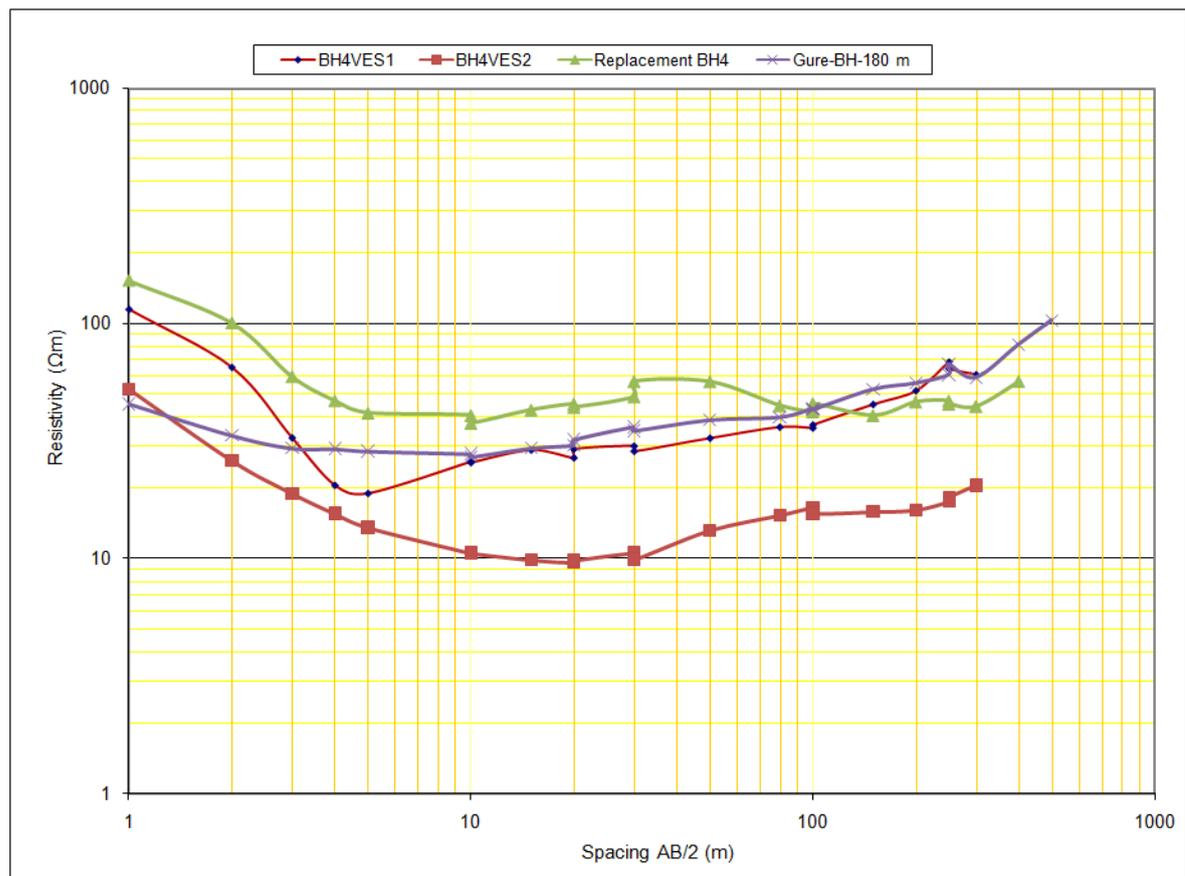
The VES from the investigated site was compared with other VES data that was already successfully drilled. Based on the resistivity pattern, all VES data was found to be very similar indicating the similarity of sub-surface geology. The interpreted result of VES soundings are summarized below tables. Layer-specific resistivity ranges (presented in the tables) are determined lithological and geological background of the area. The descriptions
