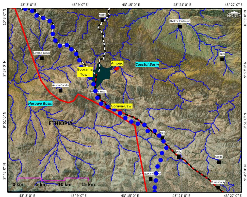
As it can be seen on the above depicted local drainage basin map of the investigated sites, Amoud areas belongs to coastal drainage basin, while Goraya-Cawl area belongs to Harawo drainage basin and is very close to the surface water divide separating between these drainage basins.
